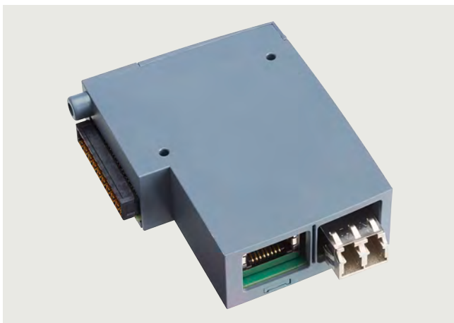
SIMATIC BA LC/RJ45 BusAdapter for use as a system-integrated media converter from copper (RJ45) to multimode glass fiber (LC).
