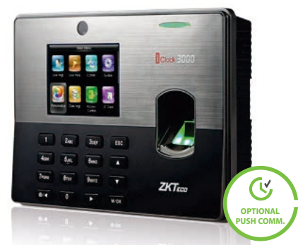
T&A and Access Control Terminal with 3,5" TFT display and Fingerprint sensor with large capacity
